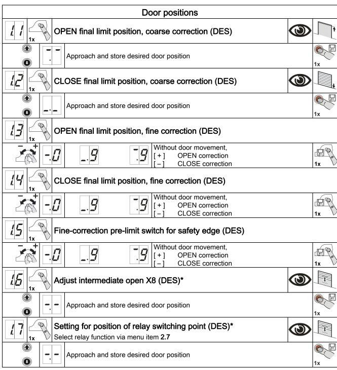
\*) Menu items **1.6** to **1.7** disappear at NES. The switching point must be adjusted via the S6 auxiliary limit switch at the drive unit.
